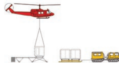
The architectural features of the Ice-Lab enable it to be transported by Bell 212 helicopter or Högglund (pictured) or inside a Twin Otter aircraft.
